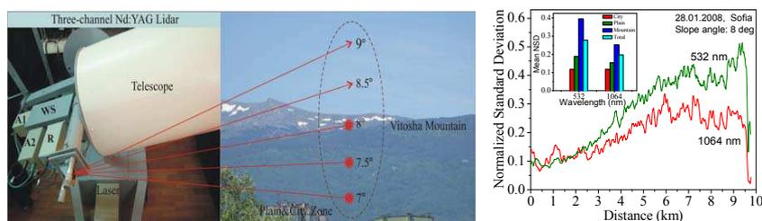
Figure 5: Schematic view of the lidar experiment over complex terrain (left) and the time-averaged range profiles of NSD and space-time averaged values of NSD over the three orographic zones (inset) for the two wavelengths of measurement (right).
