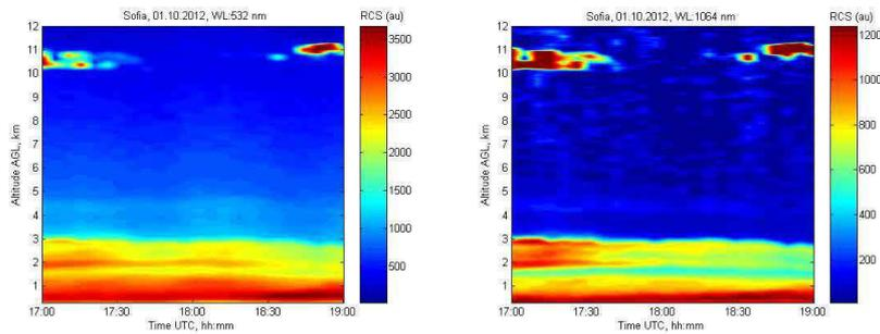
Figure 2: Time evolution of RCS measured at 532 nm (left) and 1064 nm (right) by the Nd:YAG lidar on 01.10.2012 - a Saharan dust layer seen at 1.5-3 km AGL.
