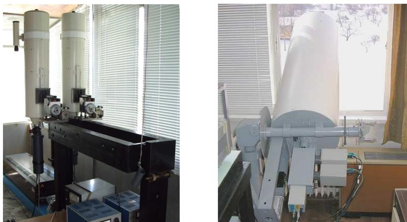
Figure 1: Photos of the CuBr-vapor laser (left) and Nd:YAG laser (right) aerosol lidars at Earlinet Sofia Station.
