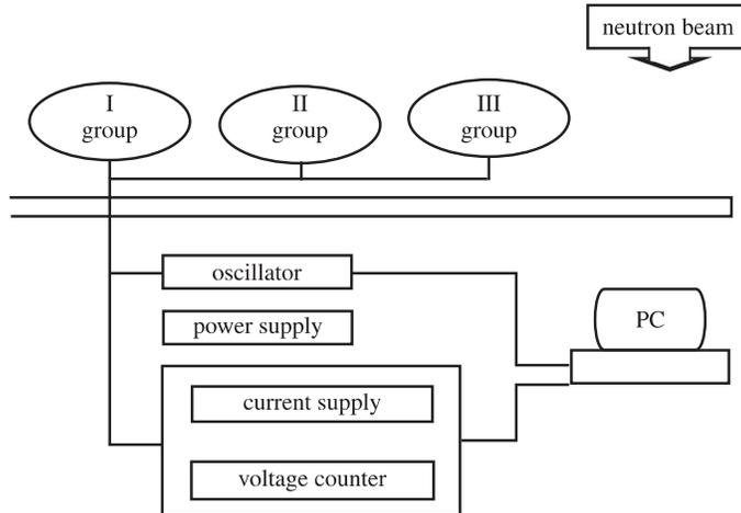
Figure 1. Fast neutron experimental setup.
