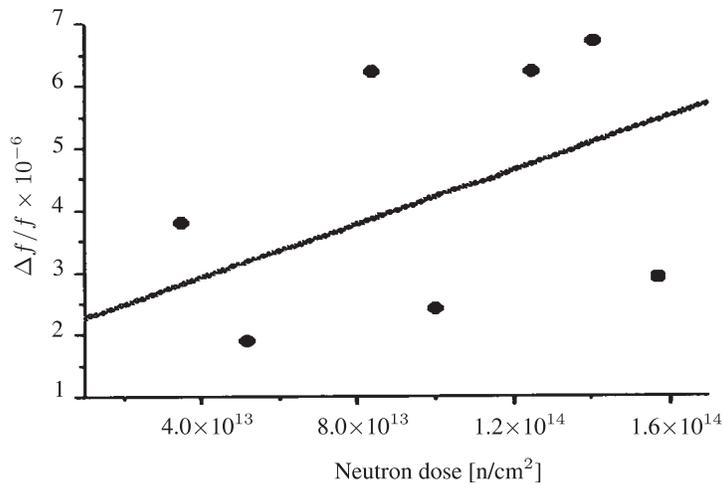
Figure 4. Influence of neutron dose on the resonant frequency at room temperature.
