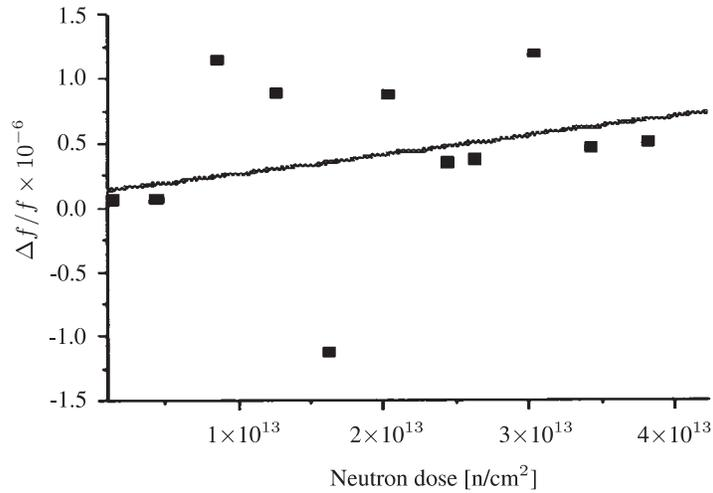
Figure 3. Influence of neutron dose on the resonant frequency at liquid nitrogen temperature.
