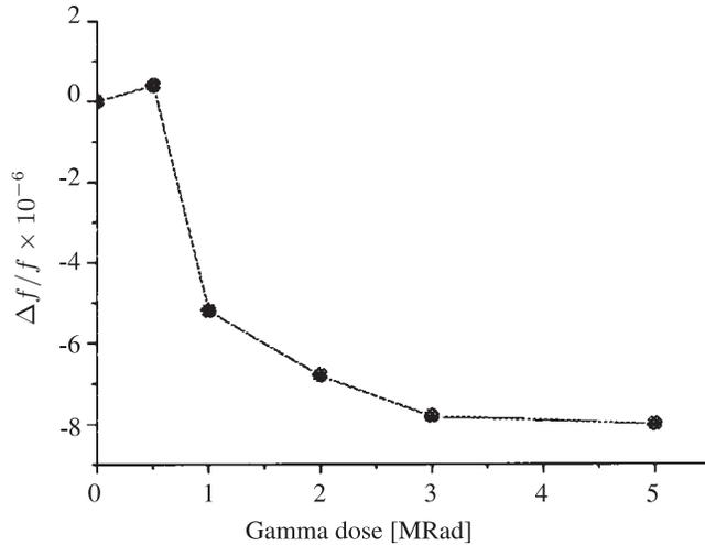
Figure 2. Influence of gamma radiation on the resonant frequency.
